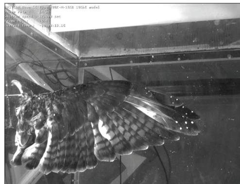
Figure 2 | A wing mounted in the wind tunnel at a gliding speed of 10 meters per second. At the top of the photos, the motor-controlled airfoils are visible, which generate upward gusts when activated. White dots along the primary feathers allow for tracking of bend, twist, and flexion by high-speed cameras.
